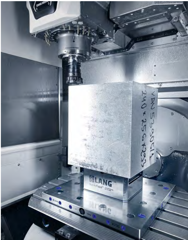
Not only highly precise, but also highly resilient. Four clamping studs are screwed directly into the workpiece, which weighs about 110 lbs.
