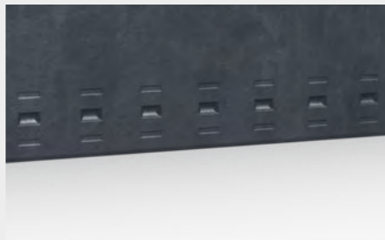
Stamping contour from tensile strength 550 N / mm 2
