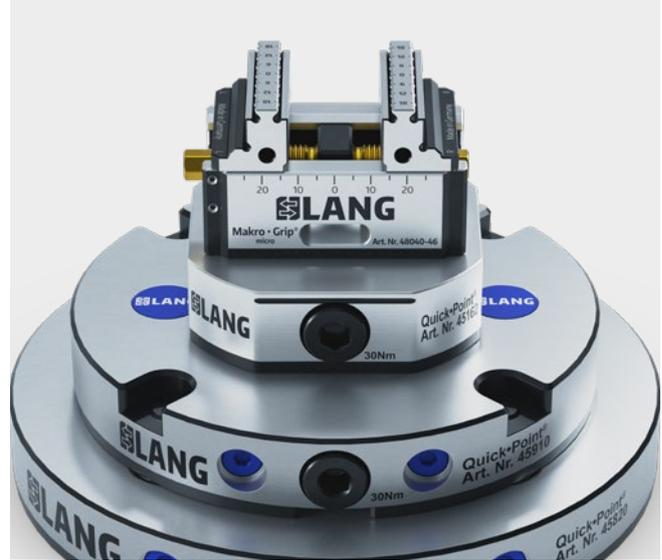
From big to very small – Even with the Quick-Point® 96 zero point clamping system, the Makro-Grip® micro can be used. This is made possible by additional adapter plates, which also provide extra accessibility in 5-sided machining.
