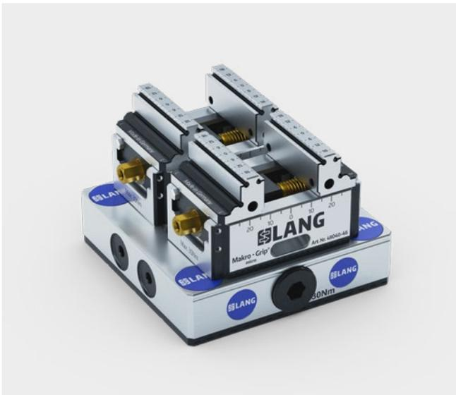
The new Quick-Point® 52 duo6 zero point plate offers three possible clamping configurations: Two Makro-Grip® 46 micro clamped side by side (as shown in the picture), one Makro-Grip® 46 micro centered or one regular Makro-Grip® 5-Axis Vise with four clamping studs.
