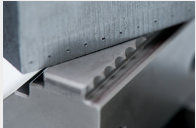
Holding teeth of a conventional vise + indentation in workpiece
