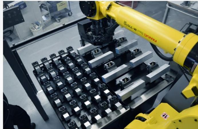
RoboTrex 96 with gripper exchange interface and different sizes of trolleys. Image: Waibel GmbH CNC-Teilefertigung
