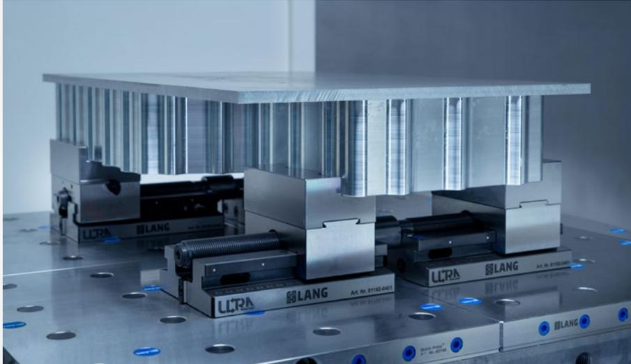
2nd OP / rear-face machining using contour jaws.
