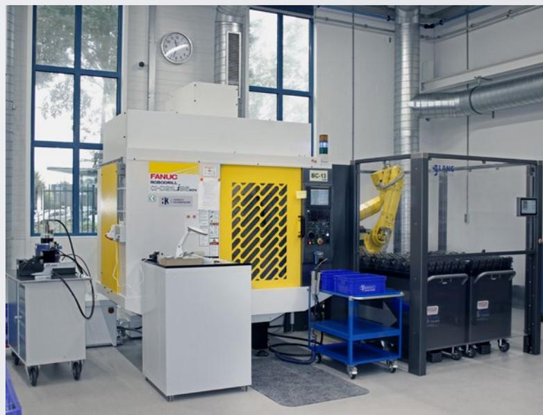
Fanuc Robodrill with RoboTrex 52 automation system. Image: Vedos Verspanende Techniek B.V.
