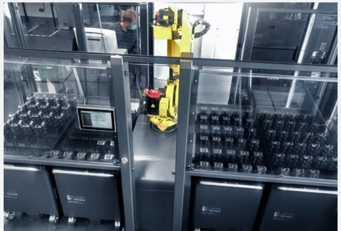
4-trolley RoboTrex 52 version attached to a DMU 60evo.
