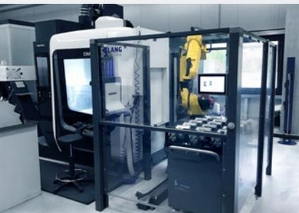
RoboTrex 52 retrofitted to a DMU 50 by DMG Mori.
